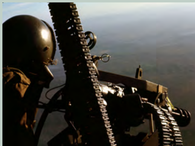
A UH-1 gunner manning a GAU-2 minigun that fired 7.62mm ammunition. (U.S. Air Force photo)
