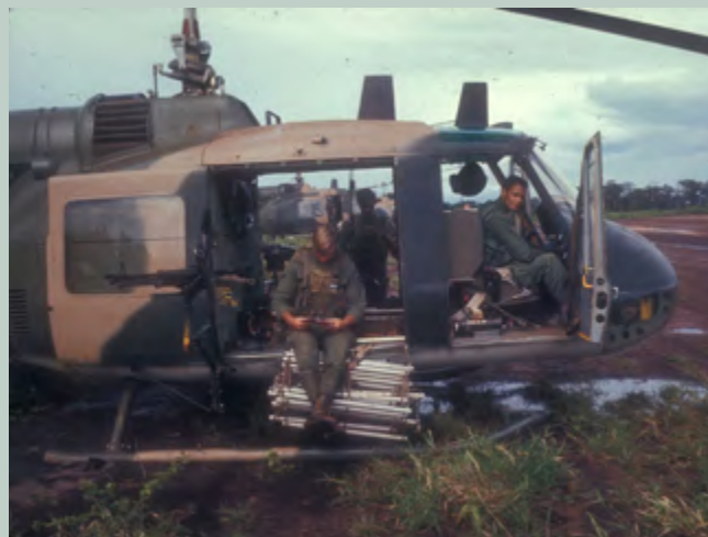
A UH-1 crew armed and ready for a covert mission. Notice the flexible ladder that could be extended to pick up personnel when the helicopter could not land. (U.S. Air Force photo)
